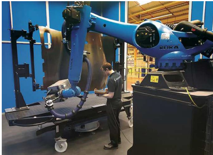
Robot IRIS : Infra red Inspection System
